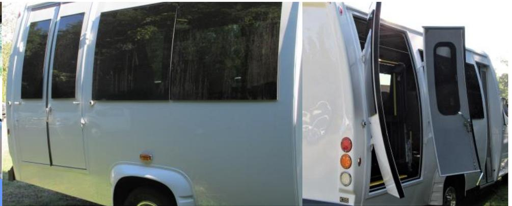
**Unique Contoured Double W/C Doors .** Matches the contour of the body without protrusions for a smooth appearance.
